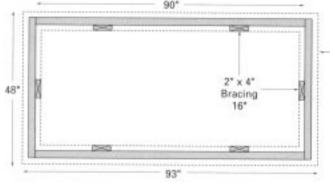
Note: Length can extend as long as desired. Use 2 x 4 braces at approximately 48\* intervals.
